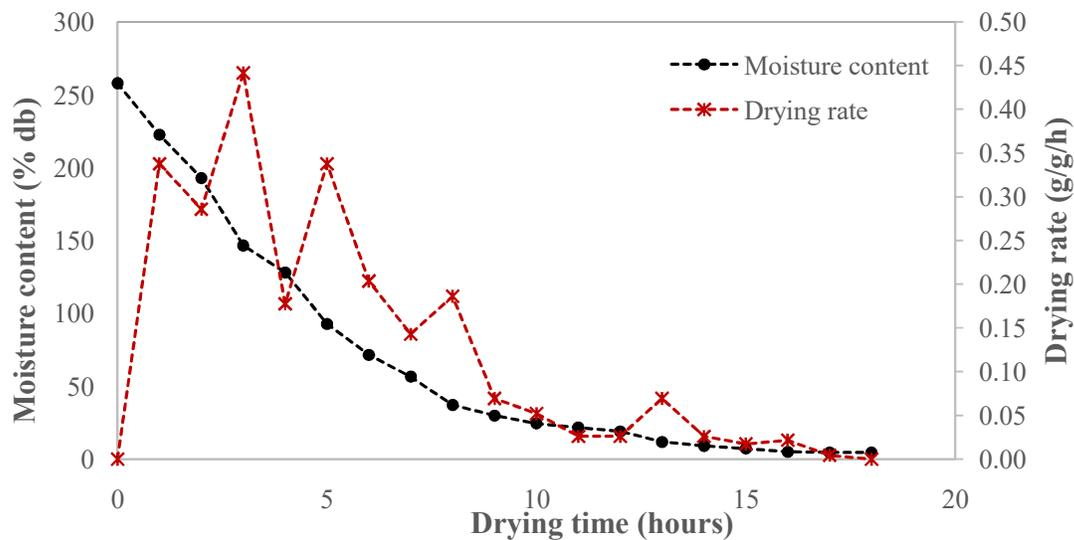
Figure 4: Drying curve and drying rate of jackfruit slices dried in a solar greenhouse dryer
