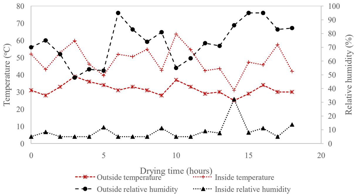
Figure 3: Variation of temperature and relative humidity in the dryer and outdoors
