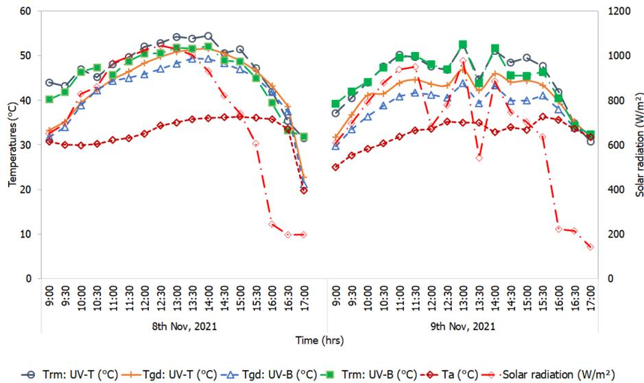
Figure 3: Variation of solar radiation, ambient temperature, and ground and room temperatures of the greenhouse solar dryers.
