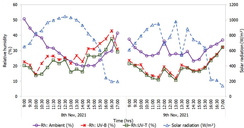
Figure 4: Variation of solar radiation, ambient relative humidity and dryer relative humidity.
