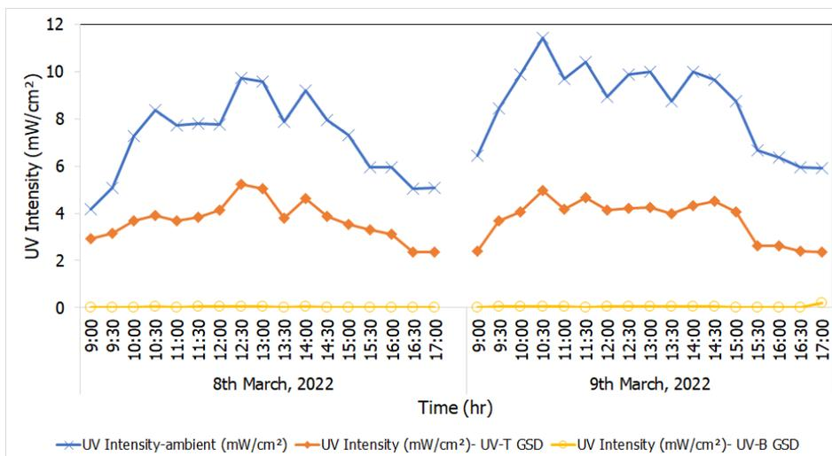
Figure 1: Profile of UV transmission intensity on two typical days
