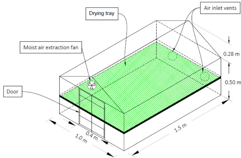
Figure 1: Schematic diagram of a greenhouse solar dryer
